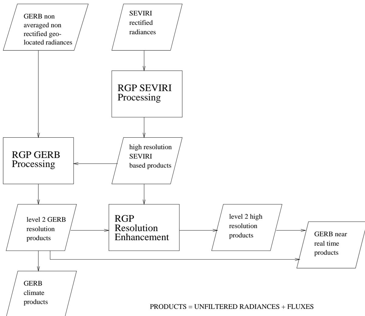
Fig 1 : Division into subsystems of the RMIB GERB Processing. The three blocks 'RGP SEVIRI Processing', 'RGP GERB Processing' and 'RGP Resolution Enhancement' are executed in sequential order.
