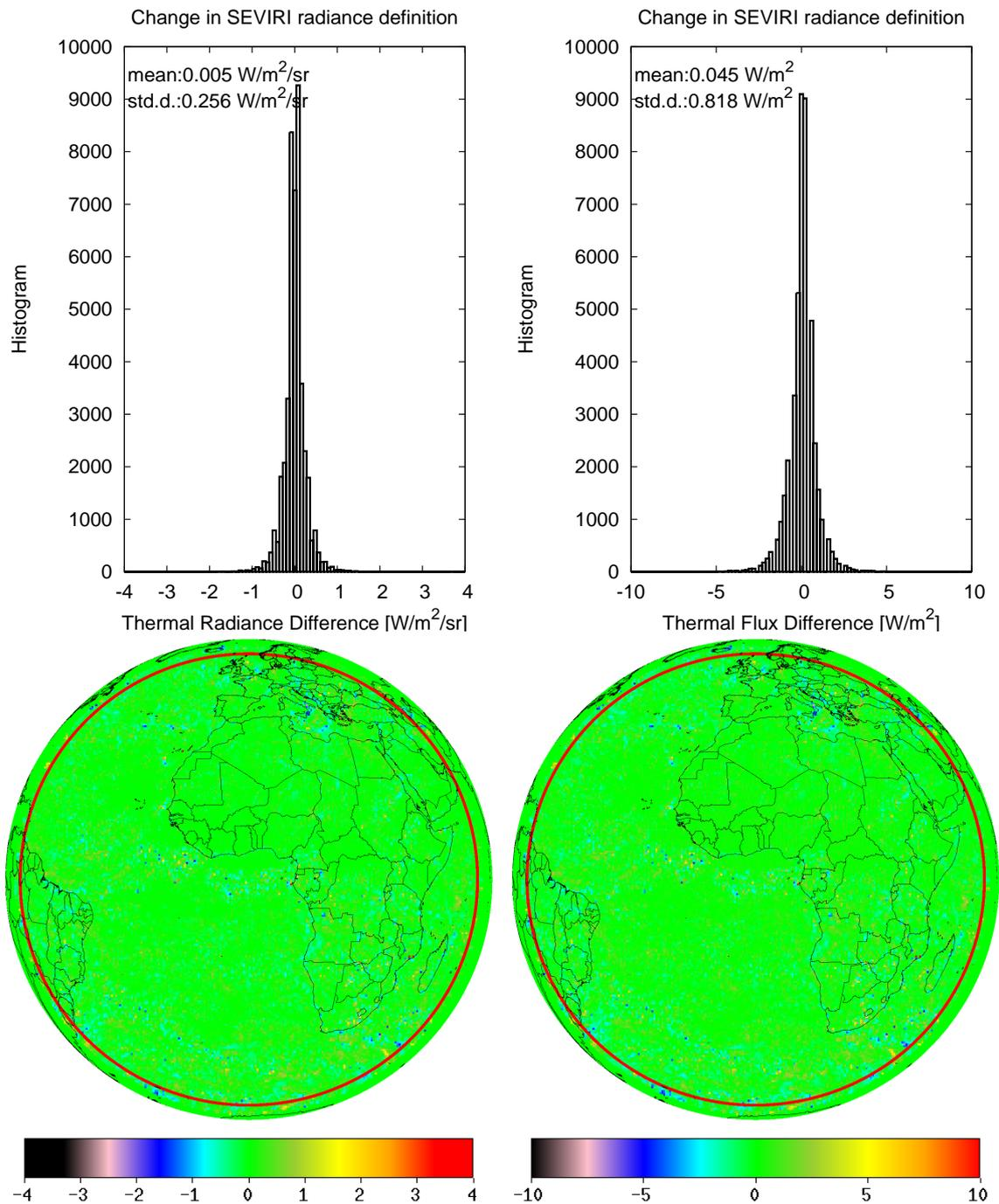
Figure 6: ARG INSTANTANEOUS THERMAL: Effect of the change in SEVIRI radiance definition on the GERB-1 emitted thermal solar (i.e. longwave) radiance (left) and flux (right). Images and histograms are averaged ARG pixel values for the 23 January 2008. The red circle indicates the VZA = 70°.
