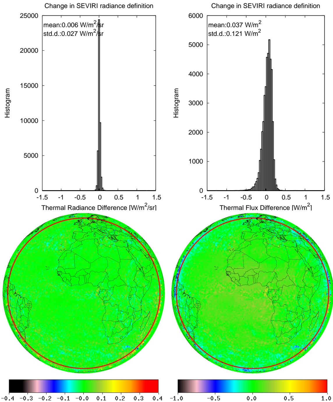
Figure 2: BARG DAILY MEAN THERMAL: Effect of the change in SEVIRI radiance definition on the GERB-1 emitted thermal solar (i.e. longwave) radiance (left) and flux (right). Images and histograms are averaged BARG pixel values for the 23 January 2008. The red circle indicates the VZA = 70°.
