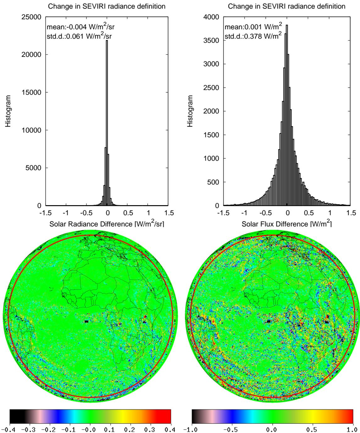
Figure 3: ARG DAILY MEAN SOLAR: Effect of the change in SEVIRI radiance definition on the GERB-1 reflected solar (i.e. shortwave) radiance (left) and flux (right). Images and histograms are averaged ARG pixel values for the 23 January 2008. The red circle indicates the VZA = 70°.
