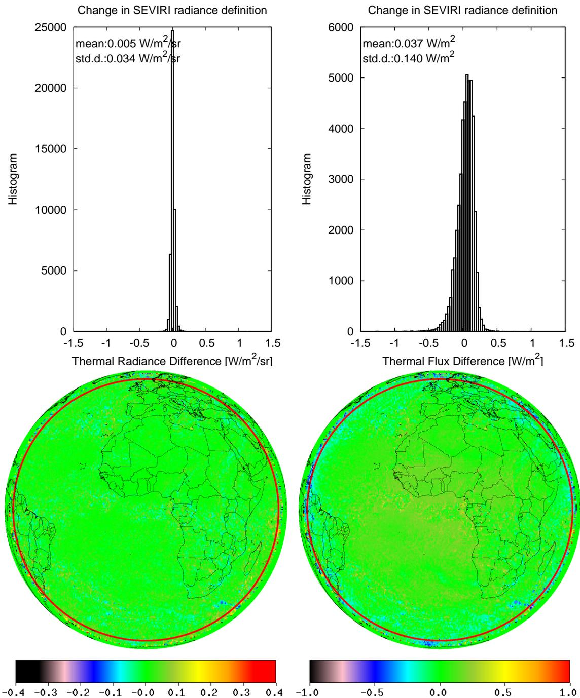
Figure 4: ARG DAILY MEAN THERMAL: Effect of the change in SEVIRI radiance definition on the GERB-1 emitted thermal solar (i.e. longwave) radiance (left) and flux (right). Images and histograms are averaged ARG pixel values for the 23 January 2008. The red circle indicates the VZA = 70°.
