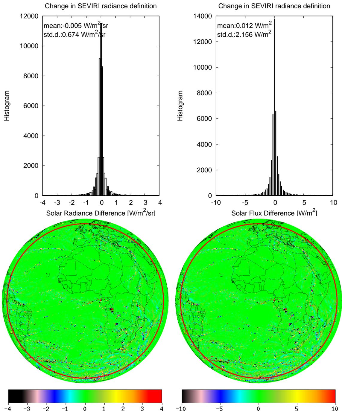
Figure 5: ARG INSTANTANEOUS SOLAR: Effect of the change in SEVIRI radiance definition on the GERB-1 reflected solar (i.e. shortwave) radiance (left) and flux (right). Images and histograms are averaged ARG pixel values for the 23 January 2008. The red circle indicates the VZA = 70°.
