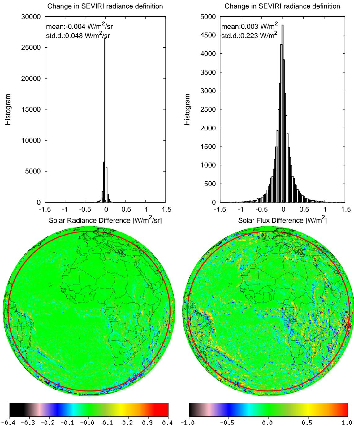
Figure 1: BARG DAILY MEAN SOLAR: Effect of the change in SEVIRI radiance definition on the GERB-1 reflected solar (i.e. shortwave) radiance (left) and flux (right). Images and histograms are averaged BARG pixel values for the 23 January 2008. The red circle indicates the VZA = 70°.
