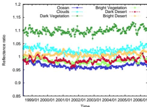
Best  $\alpha = 0.000050 \text{ days}^{-1}$  and  $\beta = 0.000105 \text{ days}^{-1} \mu\text{m}^{-1}$  which corresponds to a decrease of the spectral response curve of 1.8% per year.
