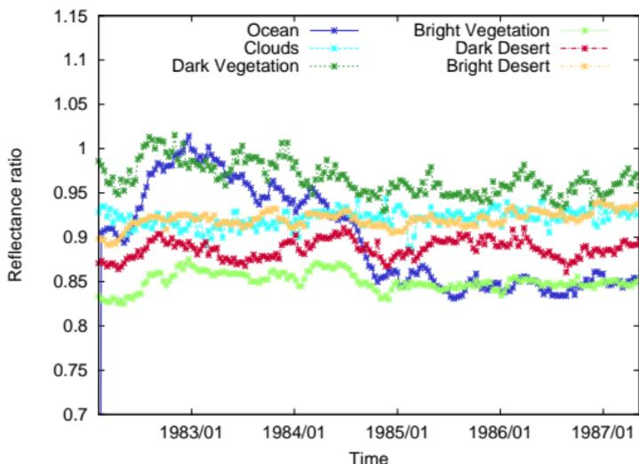
**Figure:** Time series with linear ageing model for Meteosat-2 (ageing parameter  $\alpha = 0.000035 \text{ days}^{-1}$ ).
