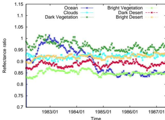
**Figure:** Time series with linear ageing model for Meteosat-7 (ageing parameter  $\alpha = 0.000035 \text{ days}^{-1}$ ,  $\beta = 0.000001 \text{ days}^{-1}$ ).
