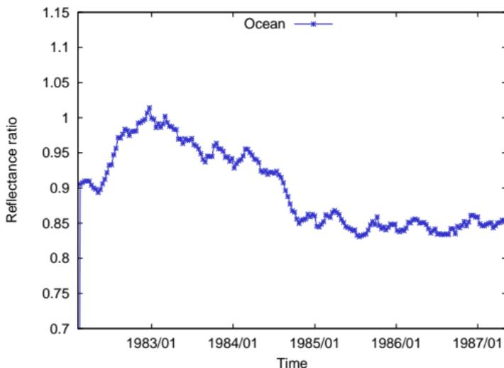
**Figure:** Ocean time series with linear ageing model for Meteosat-7 (ageing parameter  $\alpha = 0.000035 \text{ days}^{-1}$ ).
