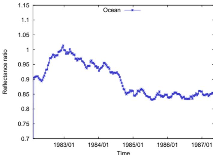
**Figure:** *Meteosat-7 ocean time series after linear ageing correction (ageing parameter  $\alpha = 0.000035 \text{ days}^{-1}$ ).*
