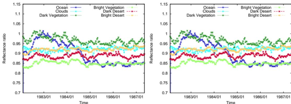
**Figure:** Time series with linear ageing model for Meteosat-2. Left figure ageing parameter  $\alpha = 0.000035 \text{ days}^{-1}$ . Right figure ageing parameters  $\alpha = 0.000035 \text{ days}^{-1}$ ,  $\beta = 0.000001 \text{ days}^{-1}$ .
