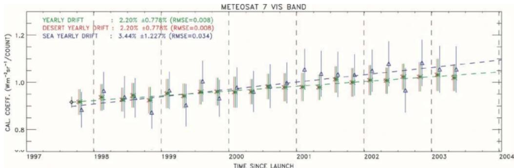
Figure: Calibration coefficient Meteosat-7 (Govaerts et al. 2004).
