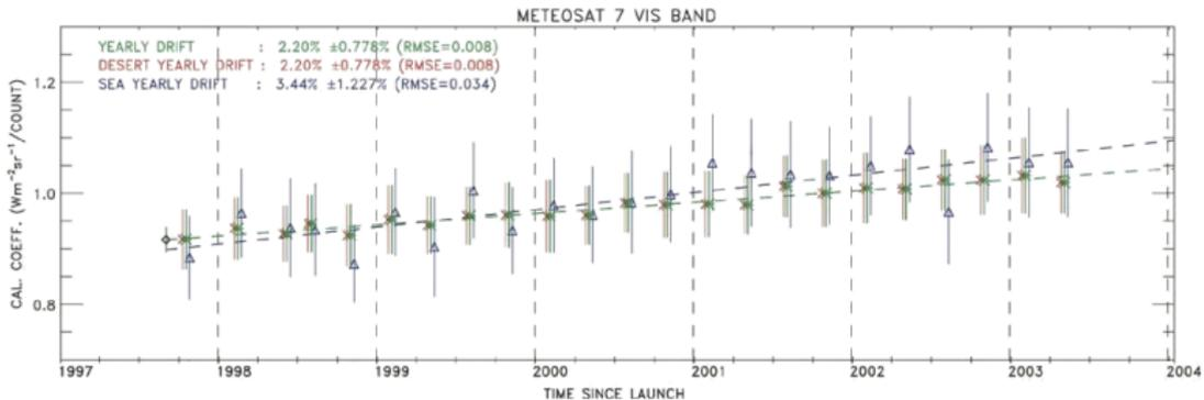
Figure : VIS calibration coefficients for Meteosat-7 (Govaerts et al. 2004).
