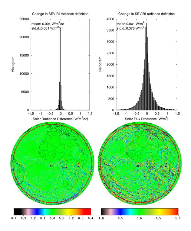
Figure 3: ARG DAILY MEAN SOLAR: Effect of the change in SEVIRI radiance definition on the GERB-1 reflected solar (i.e. shortwave) radiance (left) and flux (right). Images and histograms are averaged ARG pixel values for the 23 January 2008. The red circle indicates the VZA =  $70^{\circ}$ .
