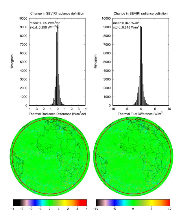
Figure 6: ARG INSTANTANEOUS THERMAL: Effect of the change in SEVIRI radiance definition on the GERB-1 emitted thermal solar (i.e. longwave) radiance (left) and flux (right). Images and histograms are averaged ARG pixel values for the 23 January 2008. The red circle indicates the VZA =  $70^{\circ}$ .
