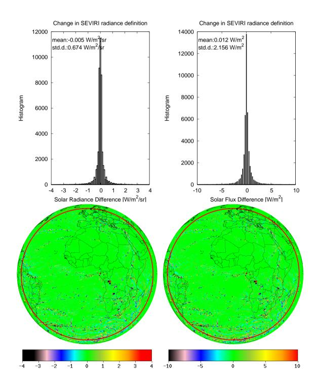
Figure 5: ARG INSTANTANEOUS SOLAR: Effect of the change in SEVIRI radiance definition on the GERB-1 reflected solar (i.e. shortwave) radiance (left) and flux (right). Images and histograms are averaged ARG pixel values for the 23 January 2008. The red circle indicates the VZA =  $70^{\circ}$ .
