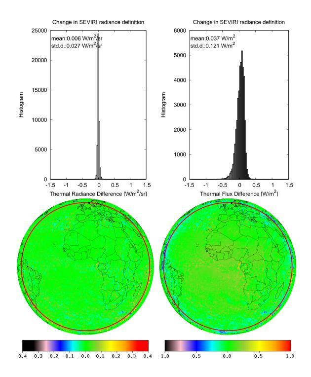
Figure 2: BARG DAILY MEAN THERMAL: Effect of the change in SEVIRI radiance definition on the GERB-1 emitted thermal solar (i.e. longwave) radiance (left) and flux (right). Images and histograms are averaged BARG pixel values for the 23 January 2008. The red circle indicates the VZA =  $70^{\circ}$ .
