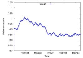
Figure: Meteosat-7 ocean time series after linear ageing correction (ageing parameter  $\alpha = 0.000035 \text{ days}^{-1}$ ).
