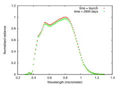
Figure: Spectral Response curve for Meteosat-7 at launch and how it could look after 2900 days.
