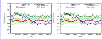
Figure: Time series with linear ageing model for Meteosat-2. Left figure ageing parameter  $\alpha = 0.000035$  days<sup>-1</sup>. Right figure ageing parameters  $\alpha = 0.000035$  days<sup>-1</sup>,  $\beta = 0.000001$  days<sup>-1</sup>.
