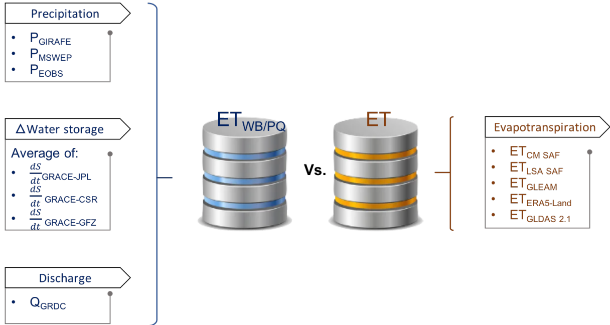
Figure 1: Schematic representation of data sources and methodologies used for estimating and comparing evapotranspiration based on the water balance method including ( ET_{WB} ) or not ( ET_{PQ} ) the change in water storage with remote sensing-based/reanalysis products.
